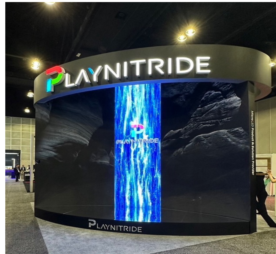
166" 5K P0.833 Waterfall Display (Seamless tiling by 324 modules) 2023 SID Best MicroLED-based Technology Award
