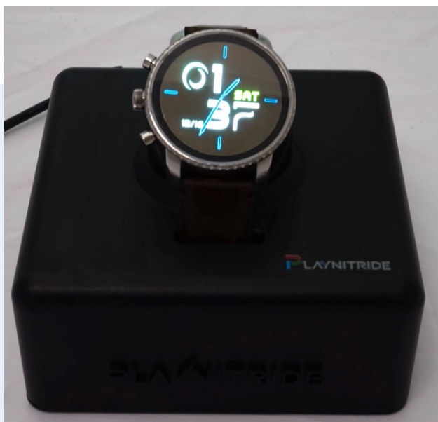
1.39" 338ppi MicroLED Circular Display
