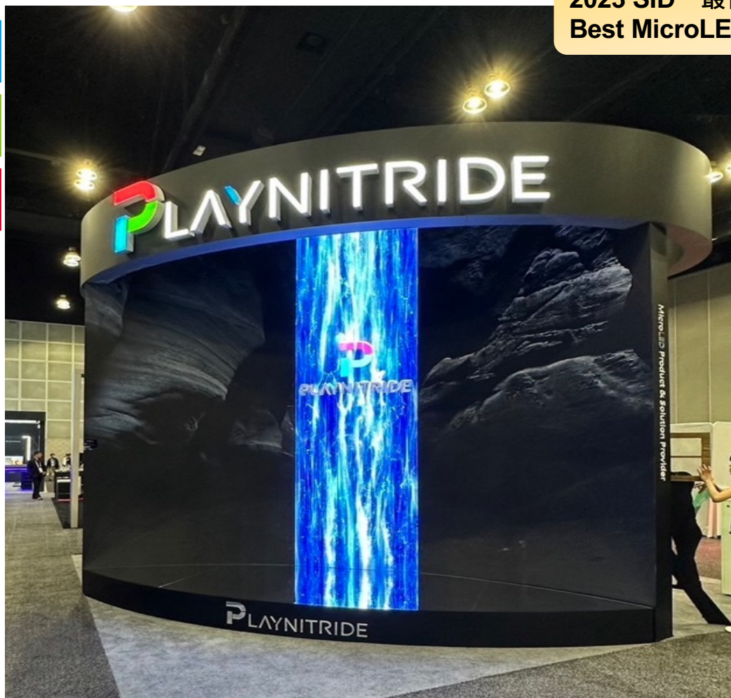
166" 5K P0.833 瀑布直立顯示看板 (Seamless tiling by 324 modules)
