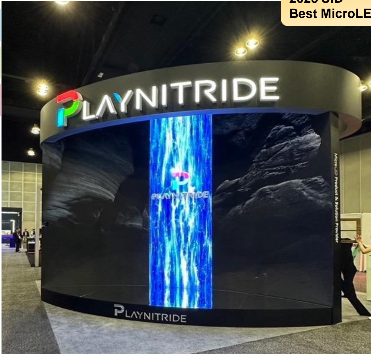
166" 5K P0.833 Waterfall Display (Seamless tiling by 324 modules)
